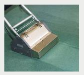
Remove the dirt-laden microcrystals using the Renovator and/or a brush vacuum cleaner.
