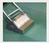
Remove loose dirt before cleaning and brush up the fiber surface layer.
