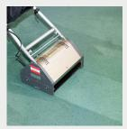
Brush in with the CRB machine. The loosened dirt will be encapsulated into microscopic crystals.
